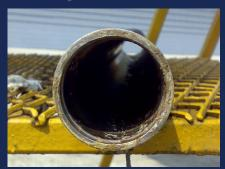
Tail section after 45 days of field testing. Sani-Tank N was also used to remove softened scale. 95% of scale was removed.
