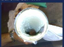
Tail section of waste line before field test. Scale buildup of 6mm thickness.
